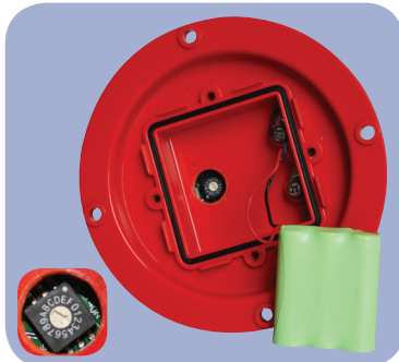
Flash characteristic is selected via internal rotary switch located in the battery compartment
