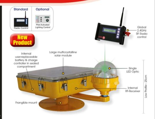
Avlite's helipad light is a solar-powered, wireless controlled, completely self-contained LED heliport light designed to meet the standards of ICAO Annex 14 Touchdown and Lift-off perimeter lights.
